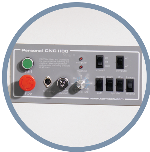
THE PCNC 1100 INTEGRATES A PC-BASED CONTROLLER WITH A HARD WIRED CONSOLE FOR SAFETY AND CONVENIENCE.
